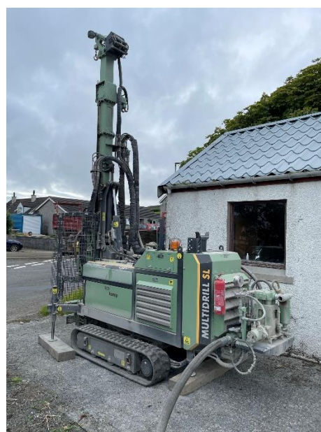
Remediation work at the Pier, soil testing and test hole drilling.
